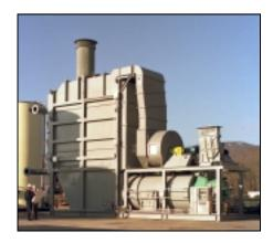
The gases are diverted upwards through the top section of the heat exchanger housing, which contains heat transfer coils. The gases pass around heat-transfer coils and heat the coils by convection.
