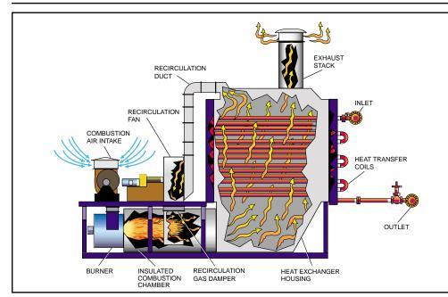
The product is heated as it flows through the heat transfer coils. The coils are heated by convection gases as they pass around the outer surfaces of the coils. The gases are recirculated to boost efficiency and to limit radiation from the burner flame.
